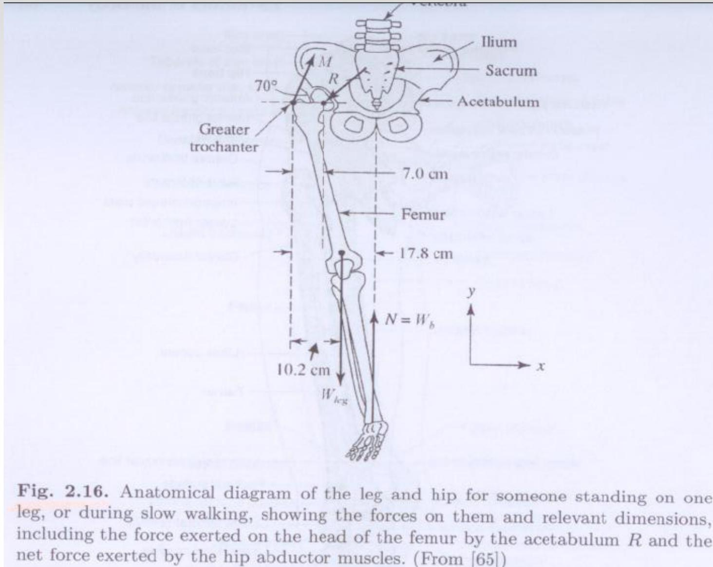
**Fig. 2.16.** Anatomical diagram of the leg and hip for someone standing on one leg, or during slow walking, showing the forces on them and relevant dimensions, including the force exerted on the head of the femur by the acetabulum  $R$  and the net force exerted by the hip abductor muscles. (From [65])
