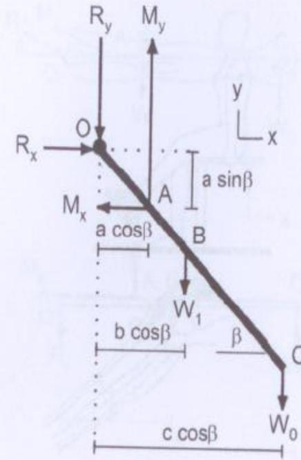
Fig. 2.24. Resolution of the forces on the lower leg in Fig. 2.23. (From [86])
