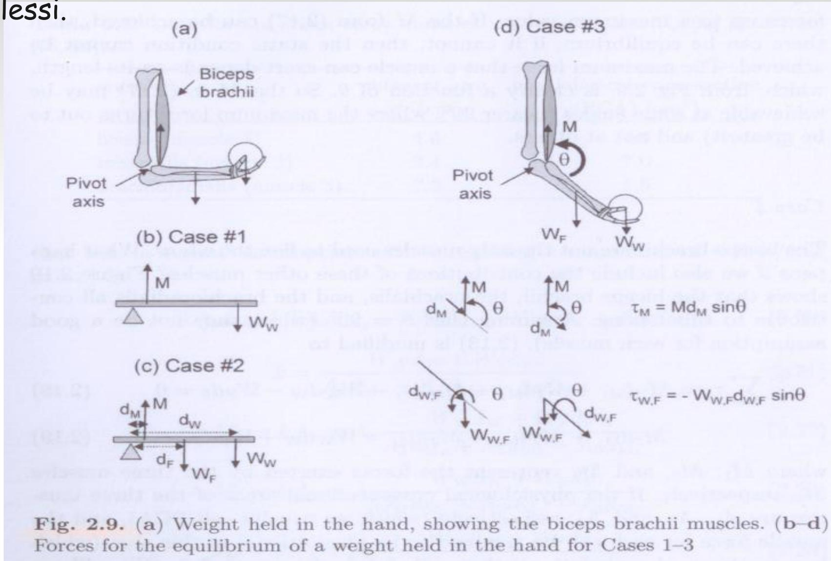
**Fig. 2.9.** (a) Weight held in the hand, showing the biceps brachii muscles. (b–d) Forces for the equilibrium of a weight held in the hand for Cases 1–3
