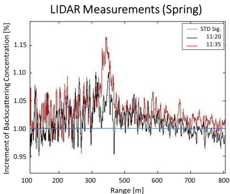
**Figure 2.** Backscattered Lidar signal in presence of smoke plume.
