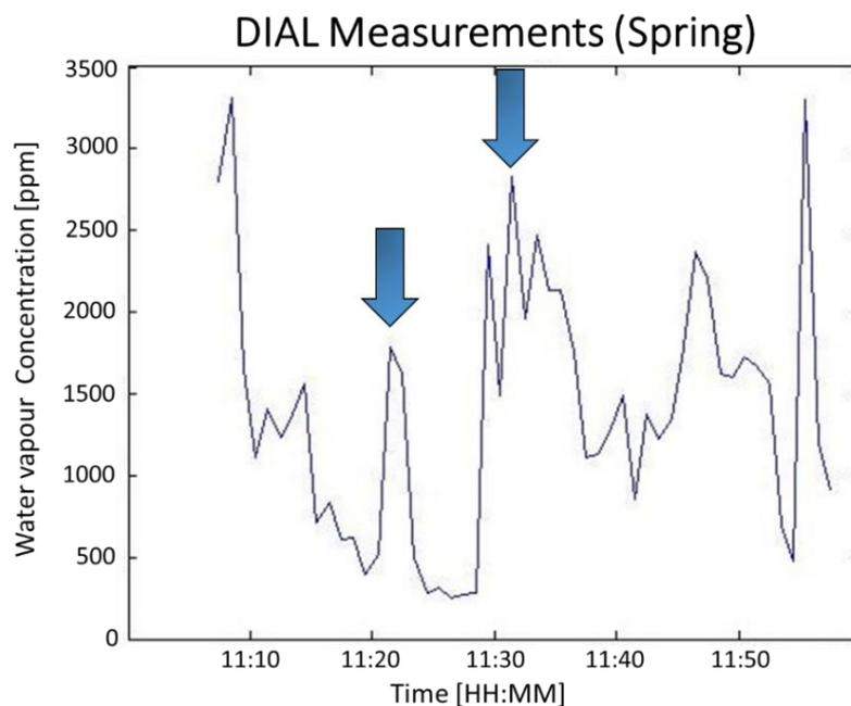
**Figure 3.** Dial signal detected in presence of fire: water vapour profile. The two peaks are quite small because a minimum amount of vegetable material has been burned.
