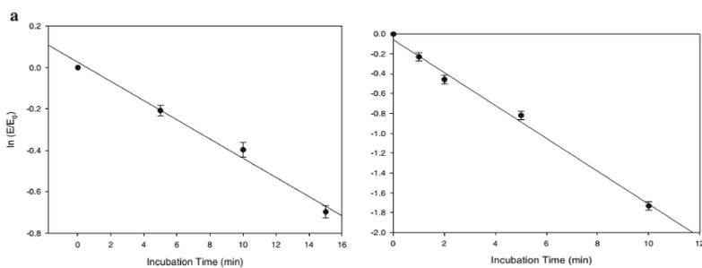
**Fig. 1** Study of  $\ln(E/E_0)$  vs incubation time using a. Acetylcholinesterase (AChE) or b. butyrylcholinesterase (BChE) biosensors. Paraoxon concentration 200 ppb. Applied potential +200 mV vs Ag/AgCl; 0.01 U AChE, 0.05 M phosphate buffer + 0.1 M KCl, pH 7.4. in the case of the AChE biosensor 1 mM acetylthiocholine chloride (ATChCl) was used, while for the BChE biosensor 5 mM butyrylthiocholine chloride (BTChCl) was used. All the values are the average of triplicate measurements.
