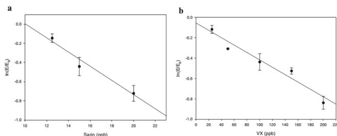
**Fig. 3** Study of  $\ln(E/E_0)$  vs inhibitor concentration. a) Sarin and b) VX using the BChE biosensor. Incubation time 10 min; applied potential + 200 mV vs Ag/AgCl; 0.01 U BChE, 5 mM BTChCl, 0.05 M phosphate buffer + 0.1 M KCl, pH 7.4. All the values are the average of triplicate measurements.
