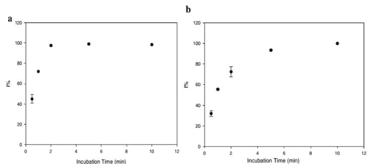
**Fig. 4** The relative inhibition of BChE activity as a function of incubation time using Sarin gas at 0.5 mg m<sup>-3</sup>, a) and 0.1 mg m<sup>-3</sup>, b) Measurement conditions 0.05 M phosphate buffer + 0.1 M KCl, pH 7.4; applied potential + 200 mv vs Ag/AgCl; 5 mM BTChCl.
