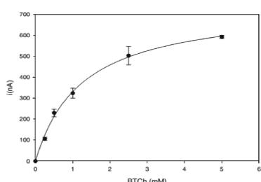
**Fig. 2** Calibration plot of butyrylthiocholine using the BChE biosensor. Applied potential + 200 mV vs Ag/AgCl; 0.01 U BChE, 0.05 M phosphate buffer + 0.1 M KCl, pH 7.4. All the values are the average of triplicate measurements.
