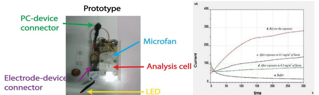
**Fig. 5** (Left) image of the prototype, (right) original recording obtained using a biosensor in 0.05 M phosphate buffer solution + 0.1 M KCl, pH 7.4. Applied potential + 200 mV vs Ag/AgCl. Signal recorded in phosphate buffer (a) and in a solution of butyrylthiocholine (5 mM) before the exposure of the biosensor to sarin gas (b) and after 1 min exposure to 0,1 mg m<sup>-3</sup> (c) and to 0.5 mg m<sup>-3</sup> (d) of Sarin gas.
